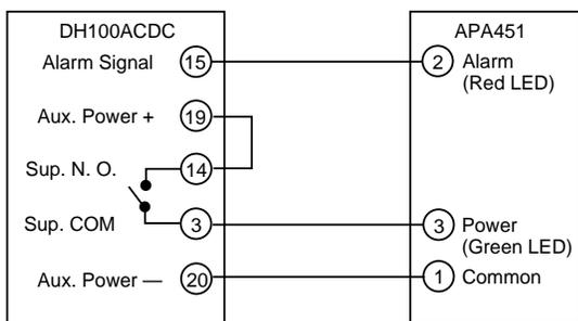
NOTE: Wiring diagram shown is for DH100ACDCLWP 4-wire duct smoke detector system equipped without a control panel.
