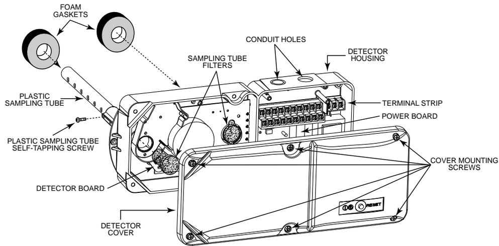
**[4] Contents Of The Duct Smoke Detector Kit**
