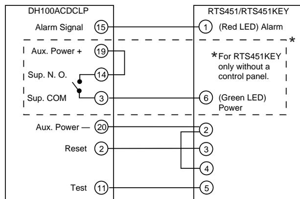
**Figure 10. Multiple fan shutdown (interconnect):**
