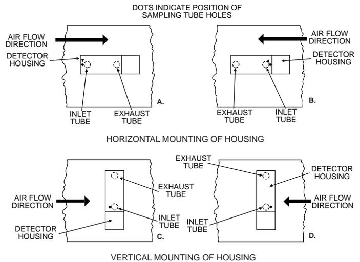
**NOTE:** Only metal sampling tubes may be used on orientations C and D.
