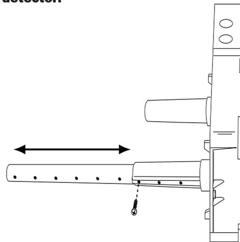
**[5.3] Secure The Detector Housing To The Duct**
