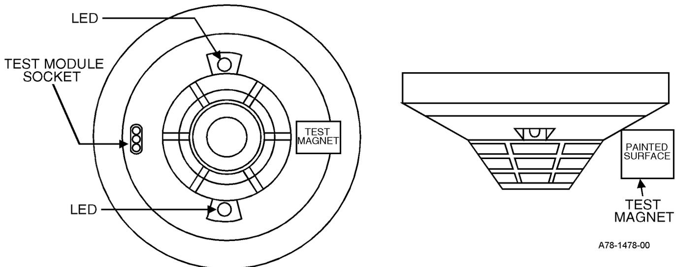
B. Test Module (System Sensor Model No. MOD400 or MOD400R)
