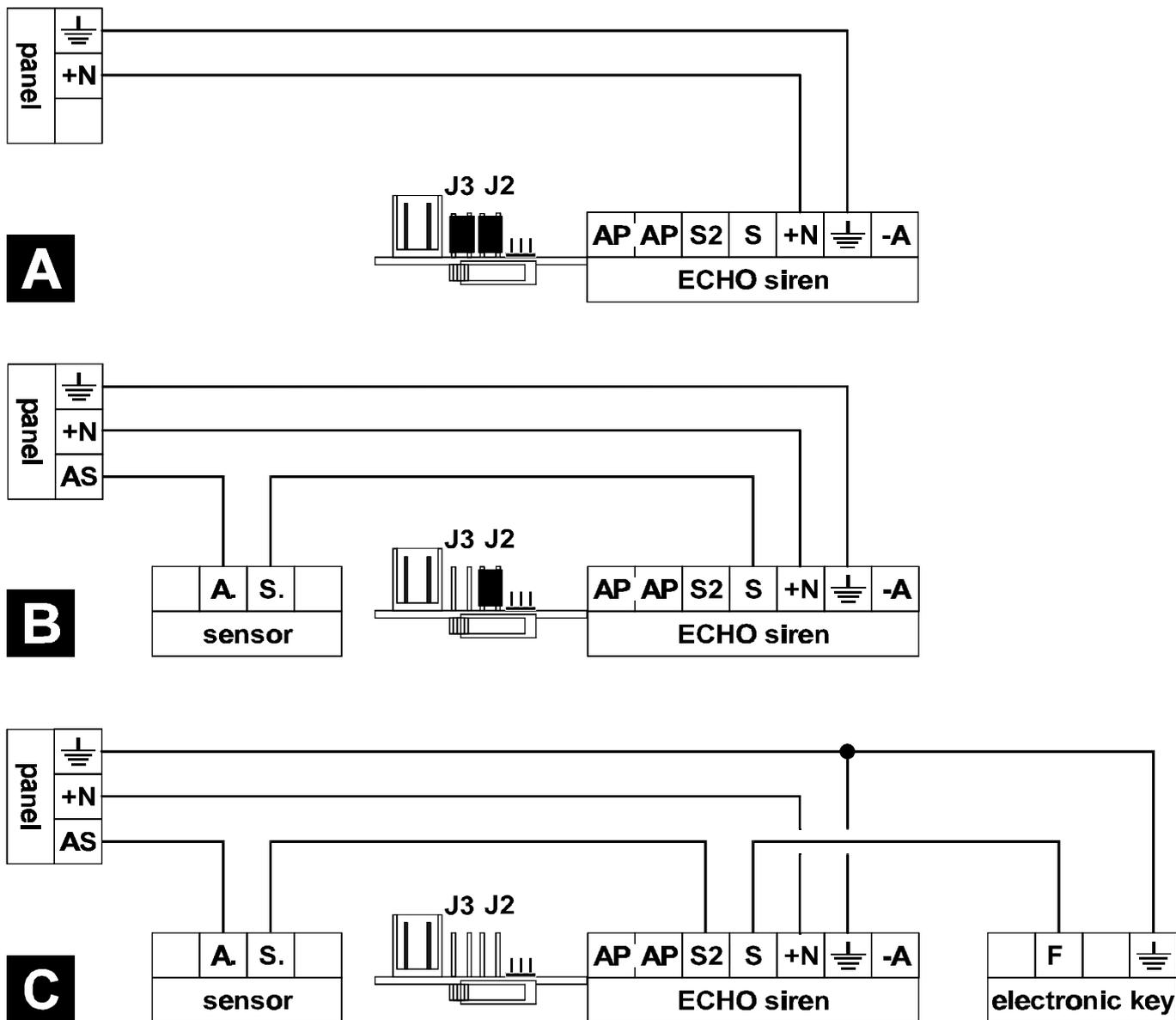
Fig. 3 - Tamper terminal connection according to the selected function mode.
