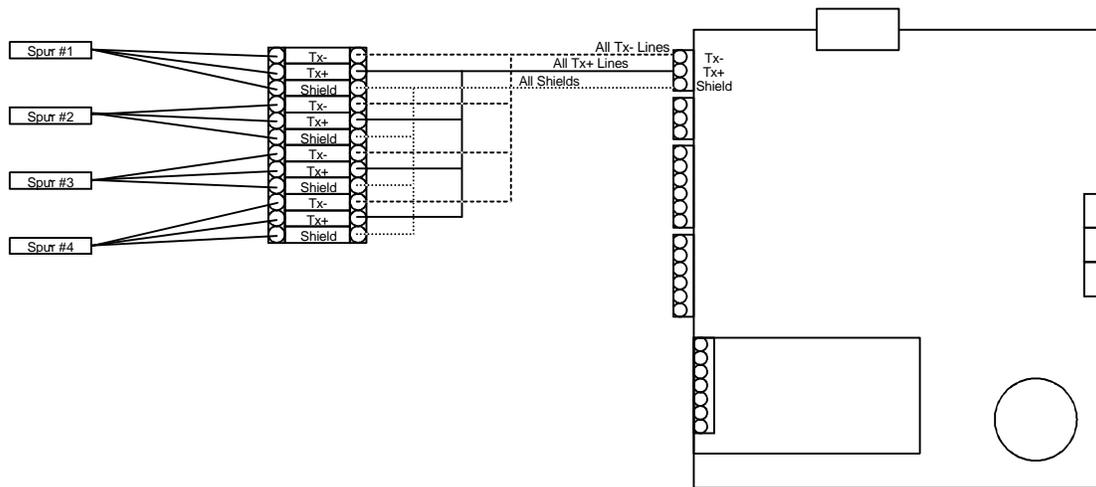
Figure 7 – Multiple Star Spurs Attached to a Master Controller
